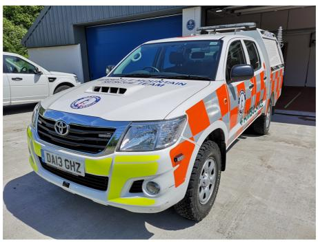
This vehicle carries up to five team members. It has a bespoke rear section with lockable roller shutter doors to accommodate a stretcher, medical supplies, climbing gear, and the team members personal rucksacks and equipment.
